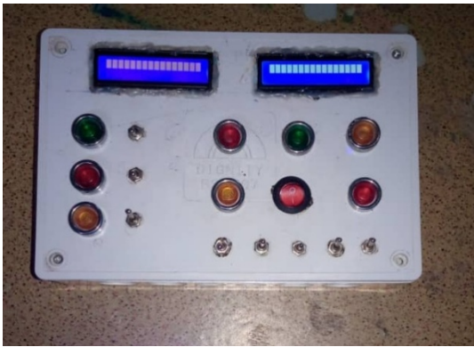
Fig. 4: The implemented hardware human machine interface model for the smart microgrid power pool system
