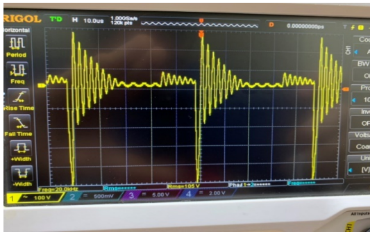
Fig. 7: The output voltage from transformer
