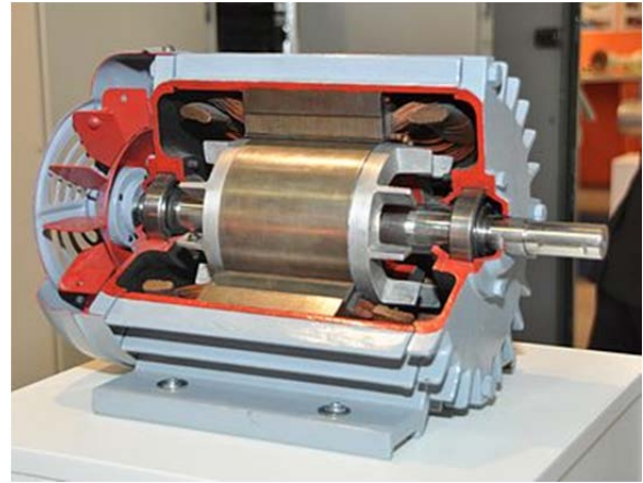
Fig. 2: Cutaway view through Induction motor [1]
