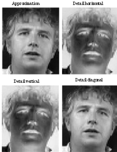
Fig. 2: One level wavelet decomposition
