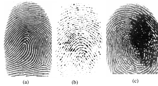
Fig. 3: a) A good quality fingerprint image; b) A poor quality fingerprint and c) A noisy fingerprint image
