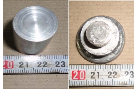
Fig. 8: Photographs of initial and deformed billets
