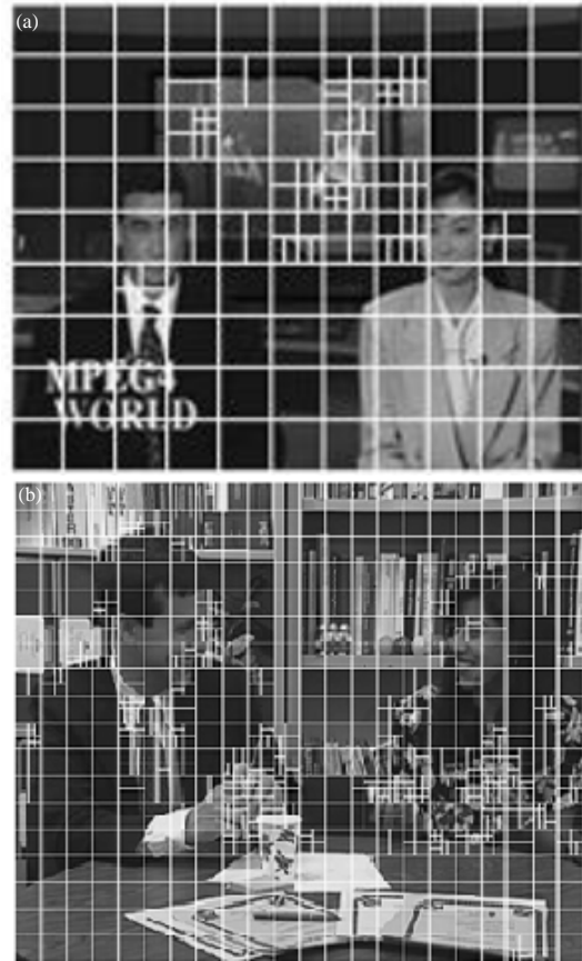
Fig. 2: Examples of block sizes chosen after inter mode search in H.264/AVC: a) News and b) Paris sequences
