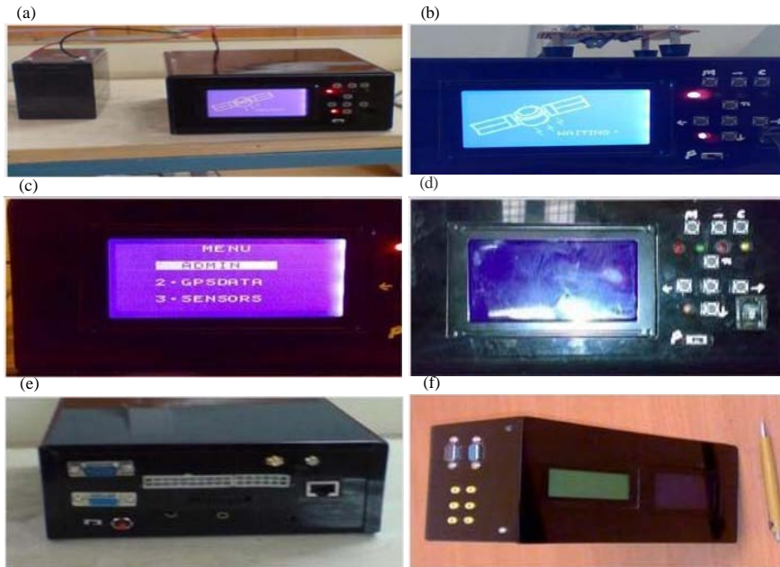
Fig. 14: ZigBee telematics box with gateway featured cloud API interface allows to collect, push information from the nodes UG and pushes it to the interface; a) GPS Galelio integrated RFID transceiver; b) Unit based on SS deadreckoning SWAPS GPS Galelio Addon card on top AoDV communication mode; c) Unit upon configured in RFID AoHC mode via tag to tag protocol on enables routing tag information without intermediate reader GW support; d) FE display button panel; e) Backend interface connections (GPS Galelio RFID-IP-HSSDIO-com) and f) Prototype-RFID-GPS Telematics with WLAN-IEEE802.11-Interface)
