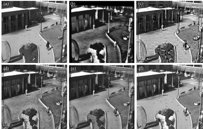
Fig. 6: OCTVBS source images (270×360, 256 levels) and fusion results; a) visible image; b) IR image and c-f) the fusion results of DWT, NSCT, Hybrid NSCT and NSCT-Fuzzy (proposed) Methods
