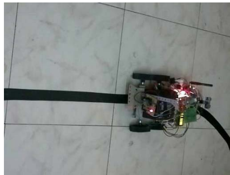
Fig. 6: Robot following line
