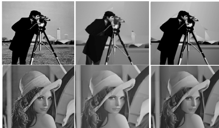
Fig. 7: Top left: original cameraman (256×256). Top center: reconstructed cameraman using the GW algorithm, 0.0625 bpp, PSNR = 22.93; top right: reconstructed cameraman using the proposed method, 0.0625 bpp, PSNR = 24.55. Bottom left: original Lena (512×512); bottom center: reconstructed Lena using the GW algorithm, 0.0625 bpp, PSNR = 28.72; bottom right: reconstructed Lena using the proposed method, 0.0625 bpp, PSNR = 29.73
