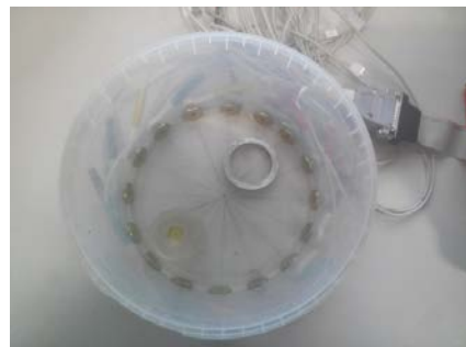
Fig. 1: Appearance of the vessel with electrodes and imperfections \Omega_1 and 2
