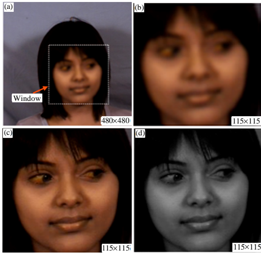
Fig. 5: a) Origin image; b) Segmented image; c) Filtered image and d) grayscaled image
