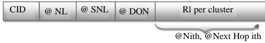
Fig. 5: Data frame encapsulation routing information; CID: Cluster Identifier, DON: Destination Ordinary Node; RI: Routing information
