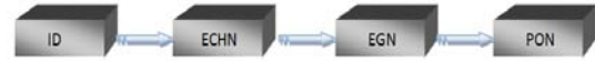
Fig. 3: CEC functioning protocol; ID: Initialization and Discovery; ECHN: Election of Cluster Head Node with highest energy; EGN: Election of Gateway Node with second highest energy; PON: Power off all other Nodes in the cluster
