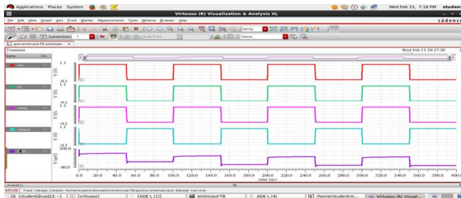
Fig. 8: The output waveform of EMTCMOS DFF 45 nm technology
