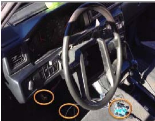
Fig. 18: The final product to control the vehicle's brake
