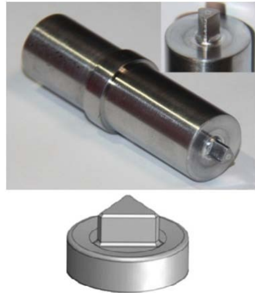
Fig. 2: Schematic and Image of beveled triangle-shaped pin
