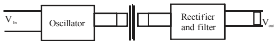
Fig. 5: Shows the basic building blocks of a High Voltage Power Supply (HVPS)
