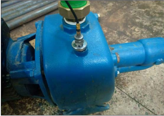
Fig. 1: Experimental test pump and sensor position
