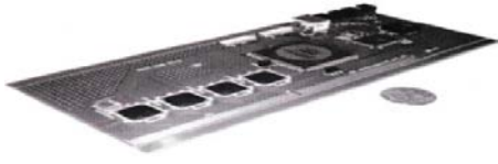
Fig. 5: The 40-ch WSFE board made with prototype WSFE ASICs. The board consists of four bare chips, a FPGA (Altera Flex) and USB controller, etc.
