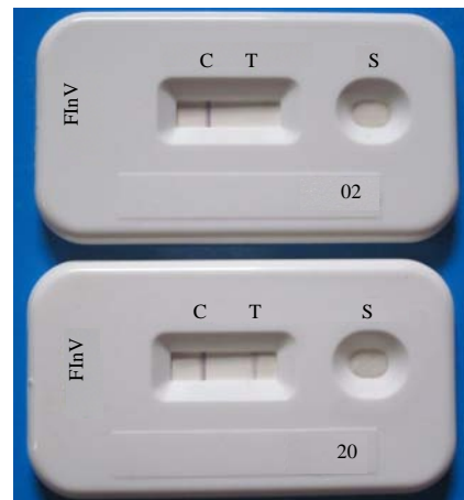
Fig. 1: Results of Feline Influenza Virus (FInV) Ag detection test showing one only band (upper one, 02) indicating negative test and showing both control and test bands (lower one, 20) indicating positive test
