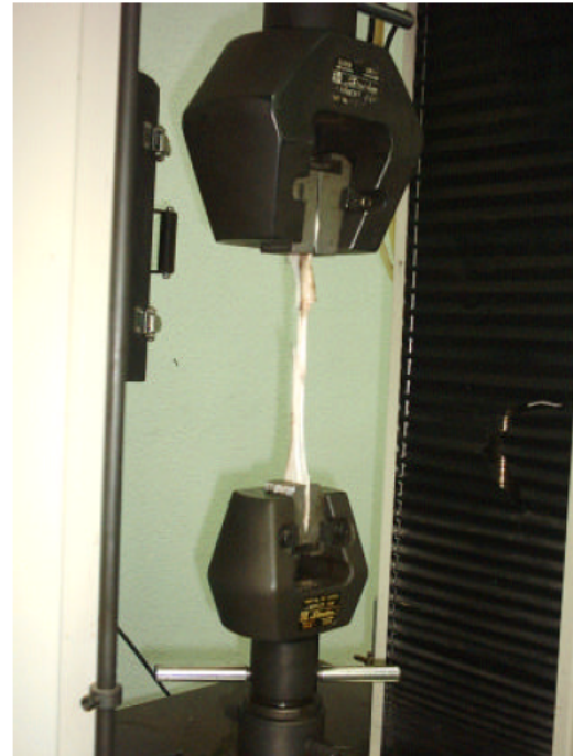
Fig. 1: Servohydraulic mechanical test system. The tendon-graft tendon unit is under the test
