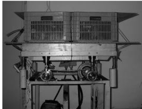
Fig 1: Road condition simulator
