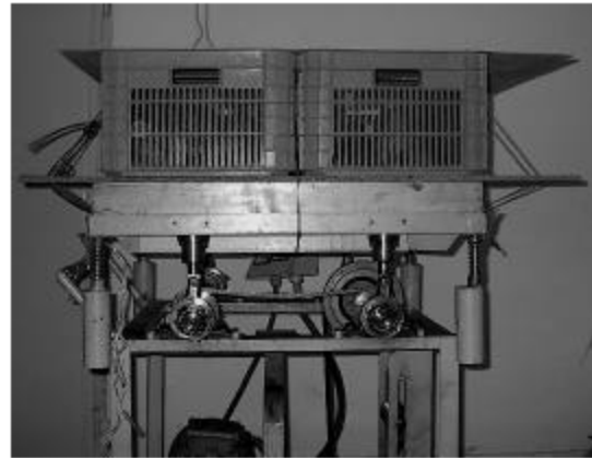
Fig 1: Road condition simulator
