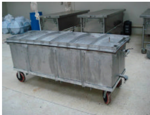
Fig. 2: A photograph showing the pressurized tank
