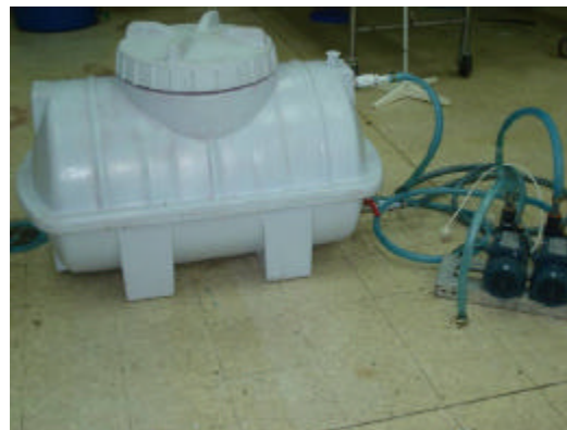
Fig. 1: A photograph showing the 250 L capacity storing tank with attached 2 pumps
