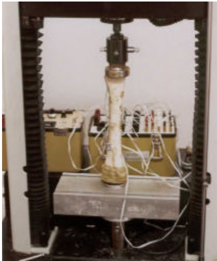
Fig. 1: Applied pressures to sample. Computer-aided Instron 4301 instrument and strain gage measurement set were used
