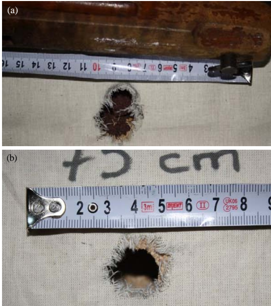
Fig. 5: a) The defect on a cotton target by shot of the modified shotgun: the range of fire is 75 cm; b) the defect on a cotton target by shot of the non-modified shotgun: the range of fire is 75 cm
