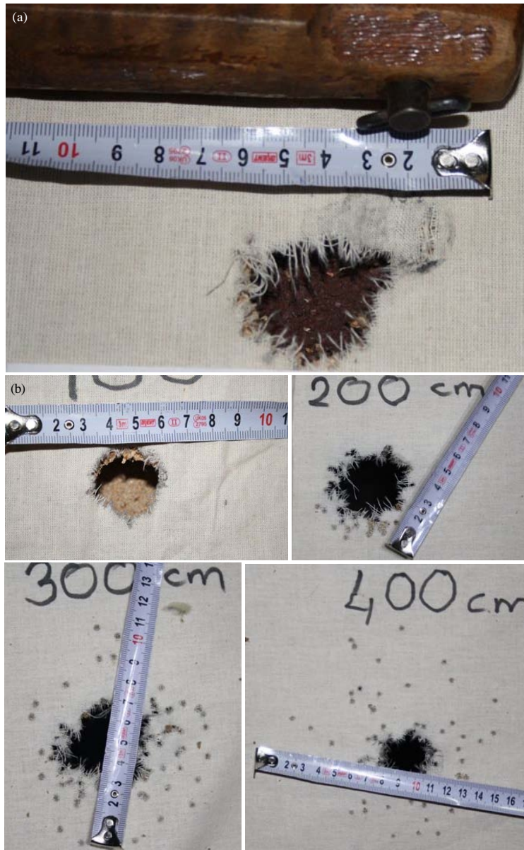
Fig. 4: a) The defect on a cotton target by shot of the modified shotgun: the range of fire is 100 cm; b) the defects on a cotton target by shots of the non-modified shotgun: the ranges of fire are 100, 200, 300 and 400 cm
