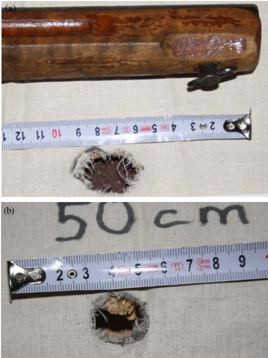
Fig. 6: a) The defect on a cotton target by shot of the modified shotgun: the range of fire is 50 cm; b) the defect on a cotton target by shot of the non-modified shotgun: the range of fire is 50 cm
