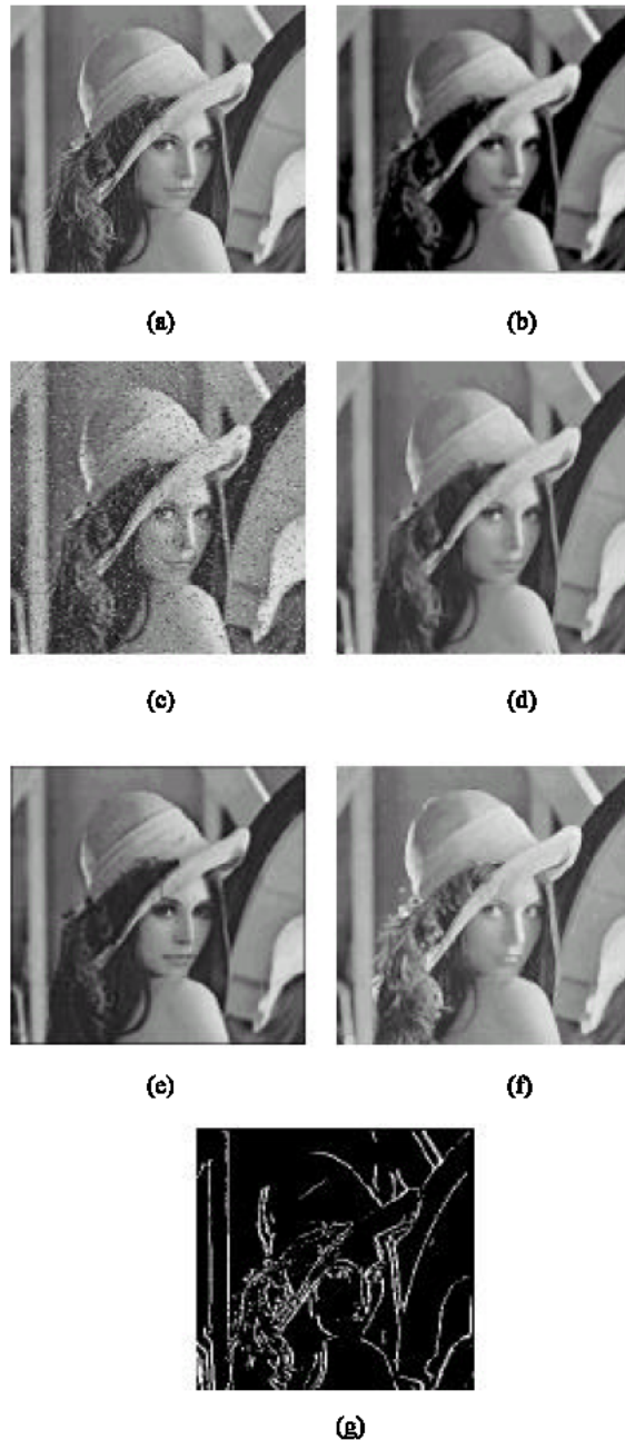
Fig. 9: (a) Original Image, (b) Gaussian convolution, (c) Salt and pepper noise, (d) Median filter, (e) Erosion, (f) Dilation, (g) Edge detection
