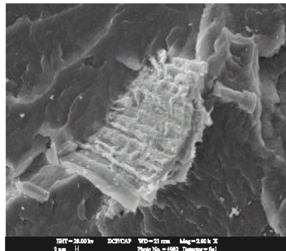
Fig. 14: SEM observation of PP/Broom Fiber/Stearic acid (70/30/1.5)
