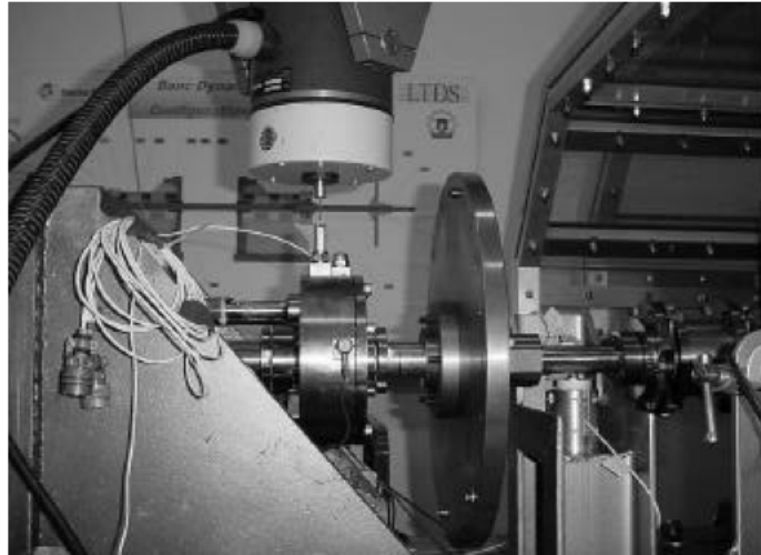
Fig. 8: Experimental setup for measuring the Campbell diagram
