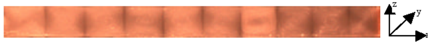
Fig. 3: Experimental streamlines observed for the Rayleigh-Bénard traditional flow in the two cases \kappa_1 and \kappa_2 , (10 rB). \Delta T=6.5 °C, Y=1.5
