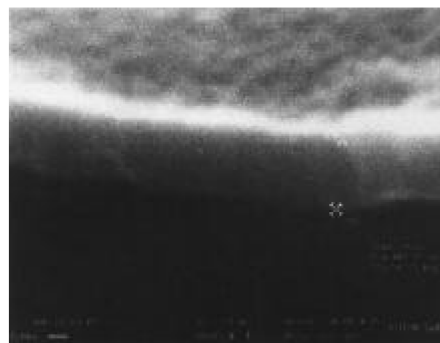
Fig. 5: Thickness of a boron layer (400 nm). Secondary electrons image
