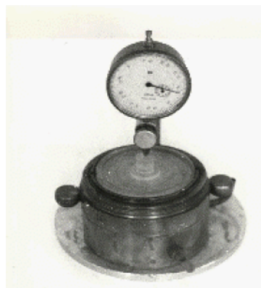
Fig. 4: Test of inflation in a free cell oedometer (without piston)
