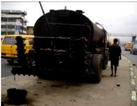
Fig. 4: A typical mobile bitumen heater at a road rehabilitation site, getting set to produce MC1/S125 at Jibowu, Lagos
