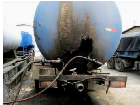
Fig. 6: Inlet and outlet valves at back of a mobile bitumen tanker
