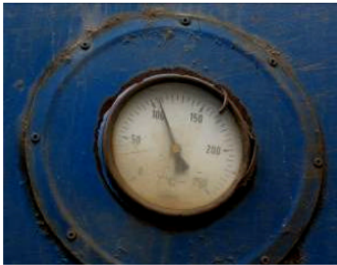
Fig. 5: A temperature dial gauge provided on the Bitumen tanker's side
