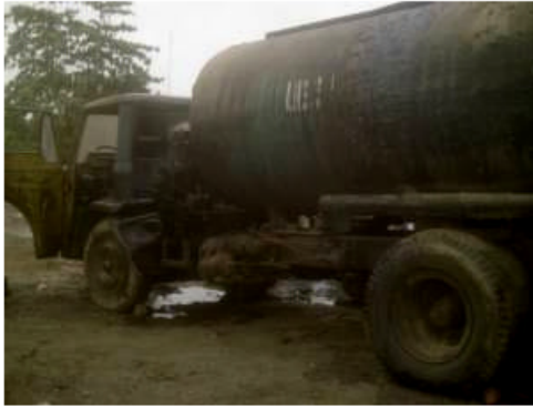
Fig. 3: Stationary bitumen heater used for the production of MC1/S125 at Lagos State Asphalt Plant
