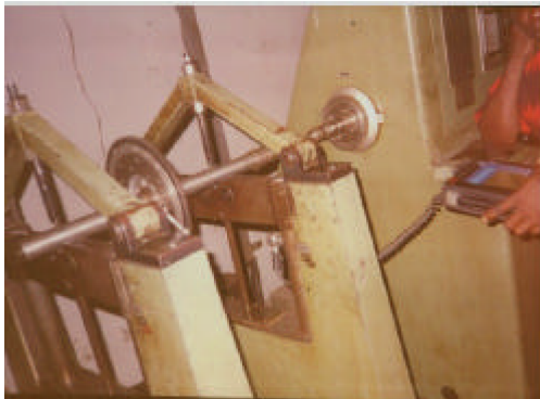
Plate 2: Taking vibration and balance data
