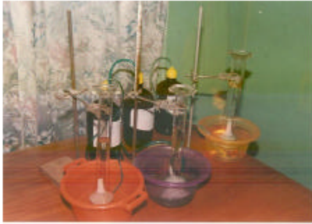
Plate 1: Experimental set up for biogas production
