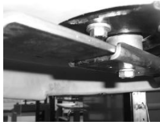
Fig. 9: Blade mounted to the bottom plate with a clear gap between them
