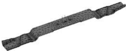
Fig. 8: The finite element mesh of a serrated cutting blade
