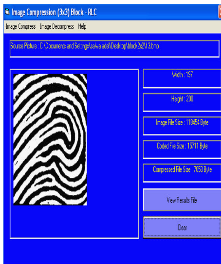
Fig. 1: Fingerprint image with (3×3) block method
