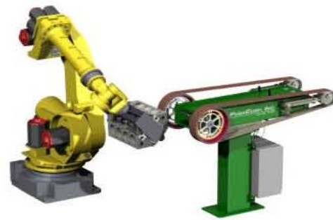
Fig. 10: Illustration of force/torque sensor in grinding Process
