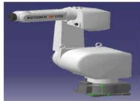
Fig. 3: Motoman DX1350N. Motoman DX1350 N Max Reach: 1355 mm, Max Payload: 35 kg Weight: 27kg, Repeatability: 0.6 mm
