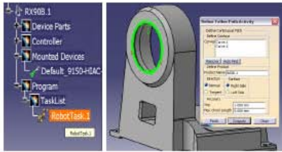
Fig 20: Snapshots windows for the selection of follow path activity under robot task
