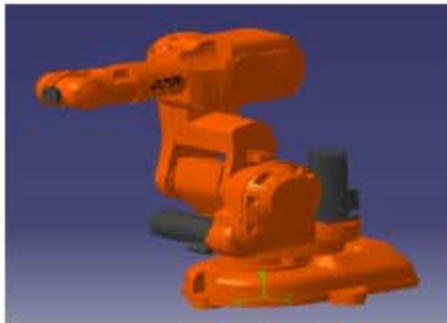
Fig 5: ABB IRB 140. IRB 140, Axis: 6, Reach: 810 mm, Payload: 5 kg Repeatability: 0.03 mm
