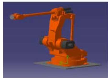
Fig. 4: Nachi SC35F. Nachi SC35 F, Max Reach: 2002 mm, Max Payload: 35 kg, Weight: 400 kg, Repeatability: 0.1 mm
