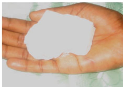
Fig. 1: A sample of soil rich in kaolinite from Pugu, Dar es Salaam-Tanzania
