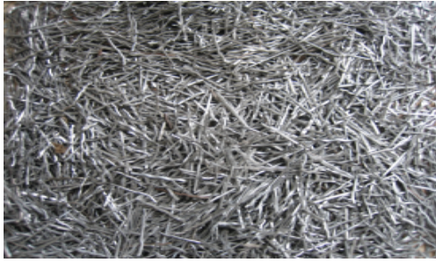
Fig. 4: Steel fiber used in the experiment
