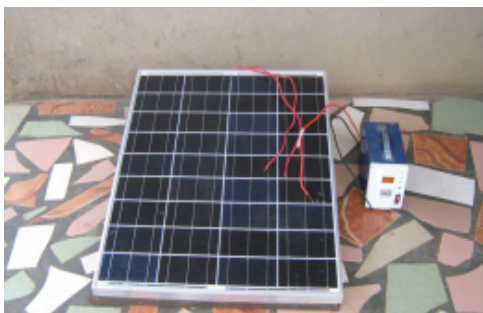
Fig. 2: Showing a stand alone 75 watts solar electric generator: the solar panel and the housed
