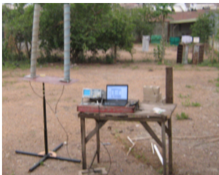
Fig. 3: The open-area experimental setup for the proposed helical antenna array
