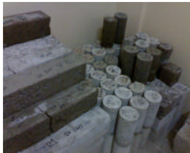
Fig. 3: Cube, cylinder and beam specimens
