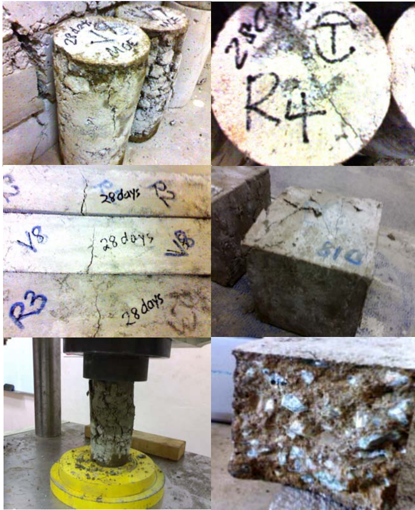
Fig. 7: Steel fibre reinforced acrylic emulsion polymer modified concrete specimens after testing
