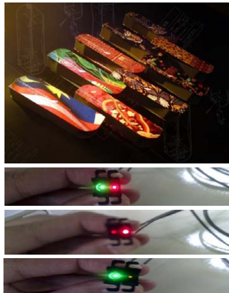
Fig. 3: Prototype of the green technology handmade 1 \times N POF demultiplexer. The device is used to split the signal to different frequency (color) which representing video and data signal (Patent Application No: PI2010700001)
