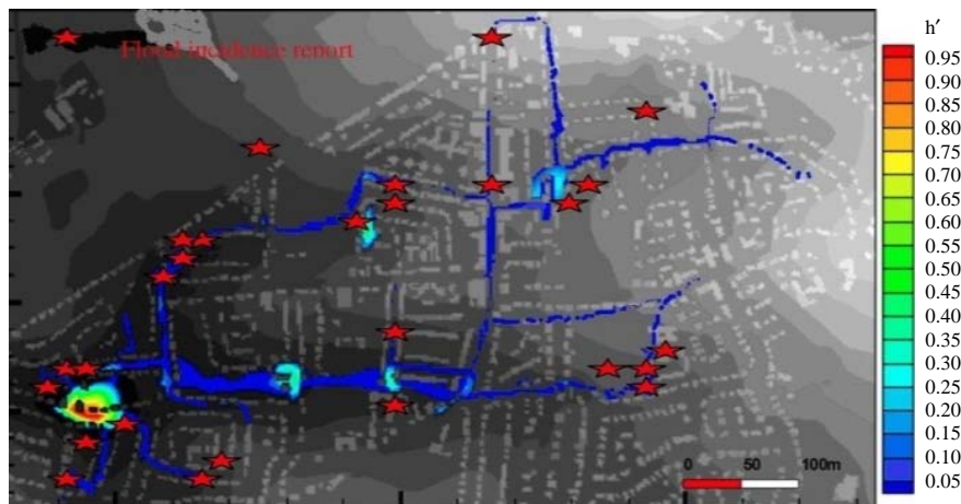
Fig. 8: Flooded nodes with flood incident reports at the case study area, West Garforth, UK
