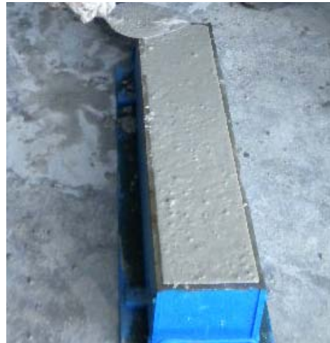
Fig. 2: Casting of beams
