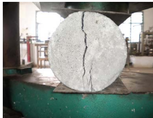
Fig. 5: Split tensile strength testing
