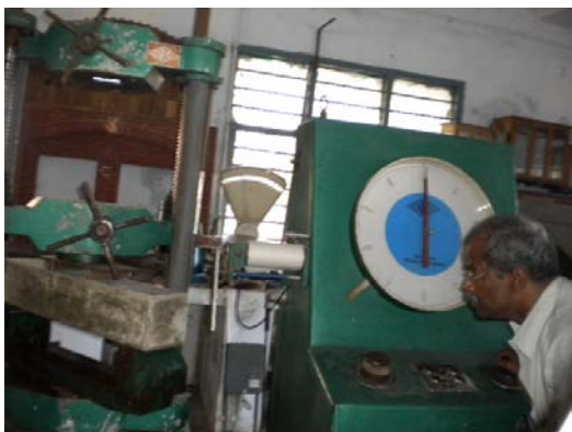
Fig. 4: Testing of beam specimens
