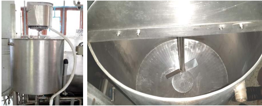
Fig. 3: Inner mixing tank with a paddle
