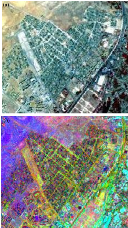
Fig. 1: Sub scene of SPOT image: a) The sub-sample of SPOT image; b) Color composite image of PCA1 and 2
