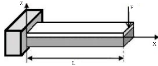
Fig. 1: Configuration of piezoelectric cantilever beam
